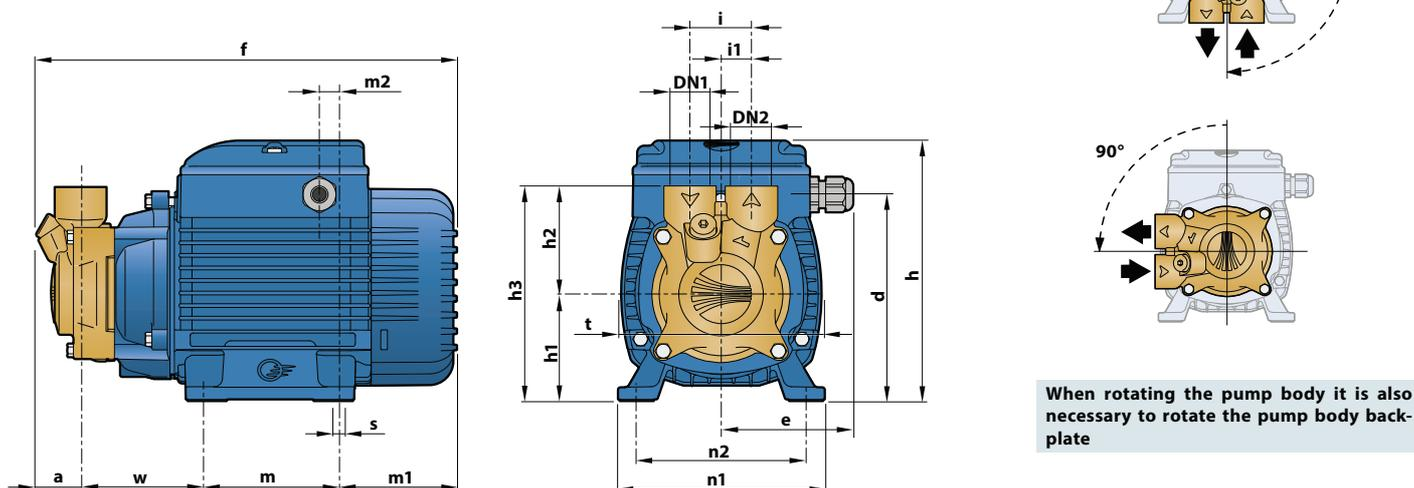
When rotating the pump body it is also necessary to rotate the pump body back-plate
